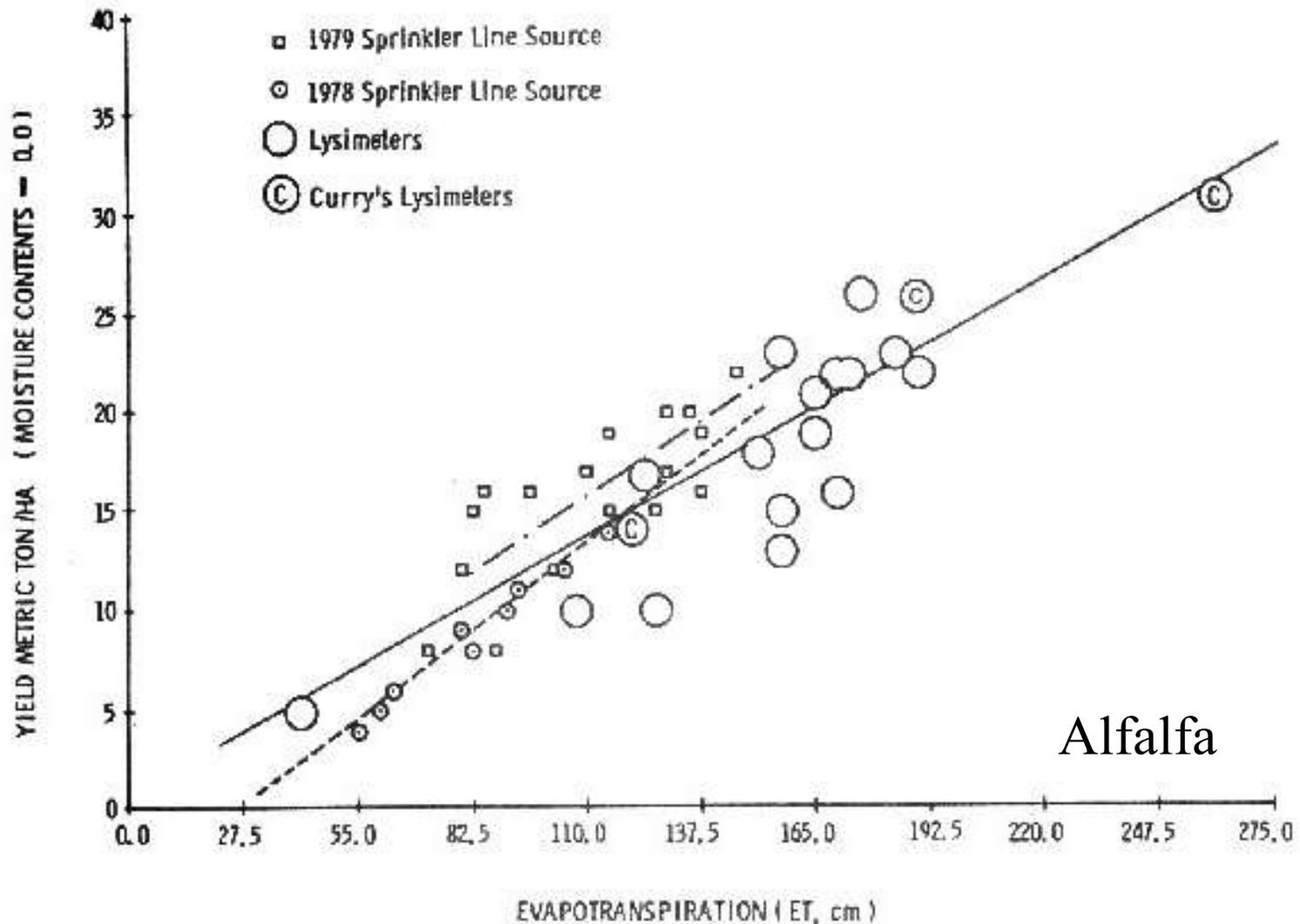
Fig. 1. Water-production function for alfalfa New Mexico.
